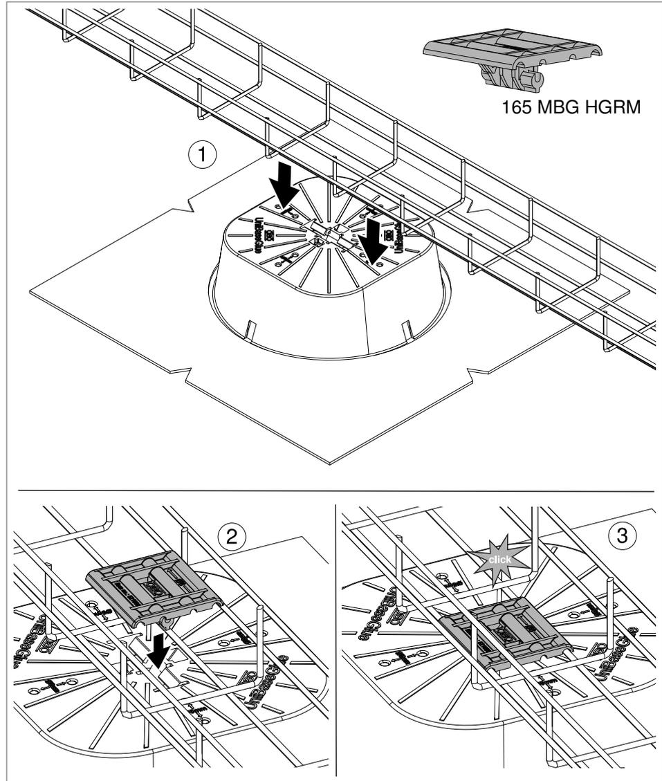
**Fig. 50:** Mounting the mesh cable tray on UniBase Glue
