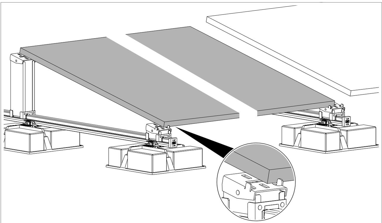
**Fig. 13:** Attaching the PV module with side fastening
