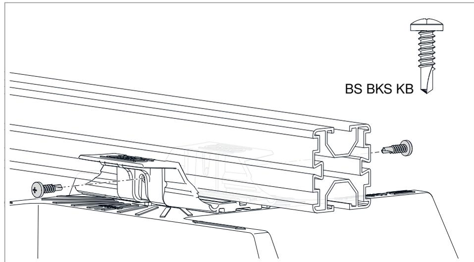
**Fig. 9:** Securing the truss profile with screws
