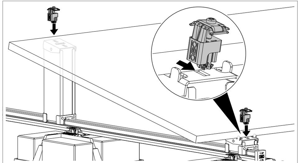
Fig. 22: Inserting the universal clamp in vertical slots
