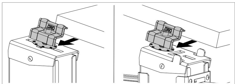
**Fig. 25:** Pushing PV module up to the end clamps
