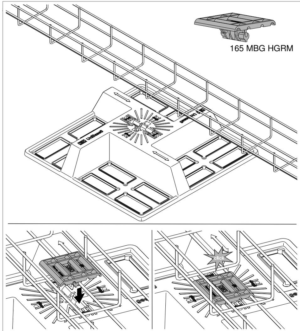
**Fig. 46:** Fastening the mesh cable tray on UniBase 6
