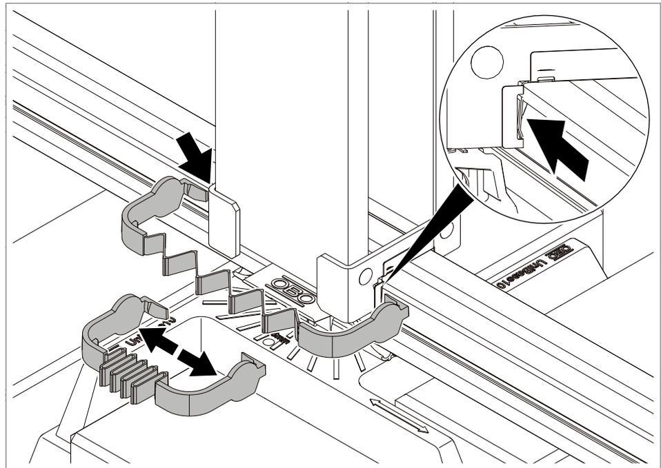
**Fig. 52:** Applying the dismantling tool
