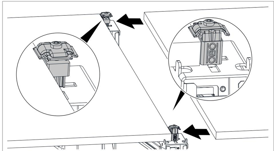
**Fig. 20:** Inserting the universal clamp in the slot
