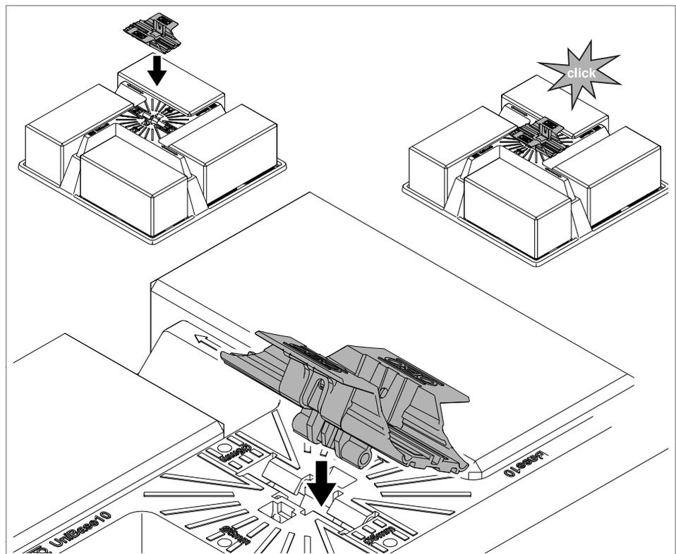
**Fig. 6:** Inserting adapters
