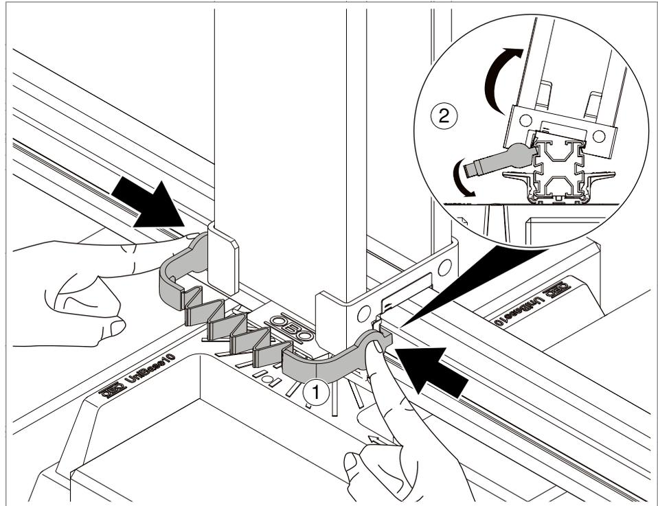
**Fig. 53:** Removing the support
