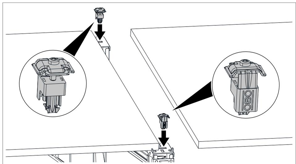
**Fig. 19:** Inserting the universal clamp in the slot
