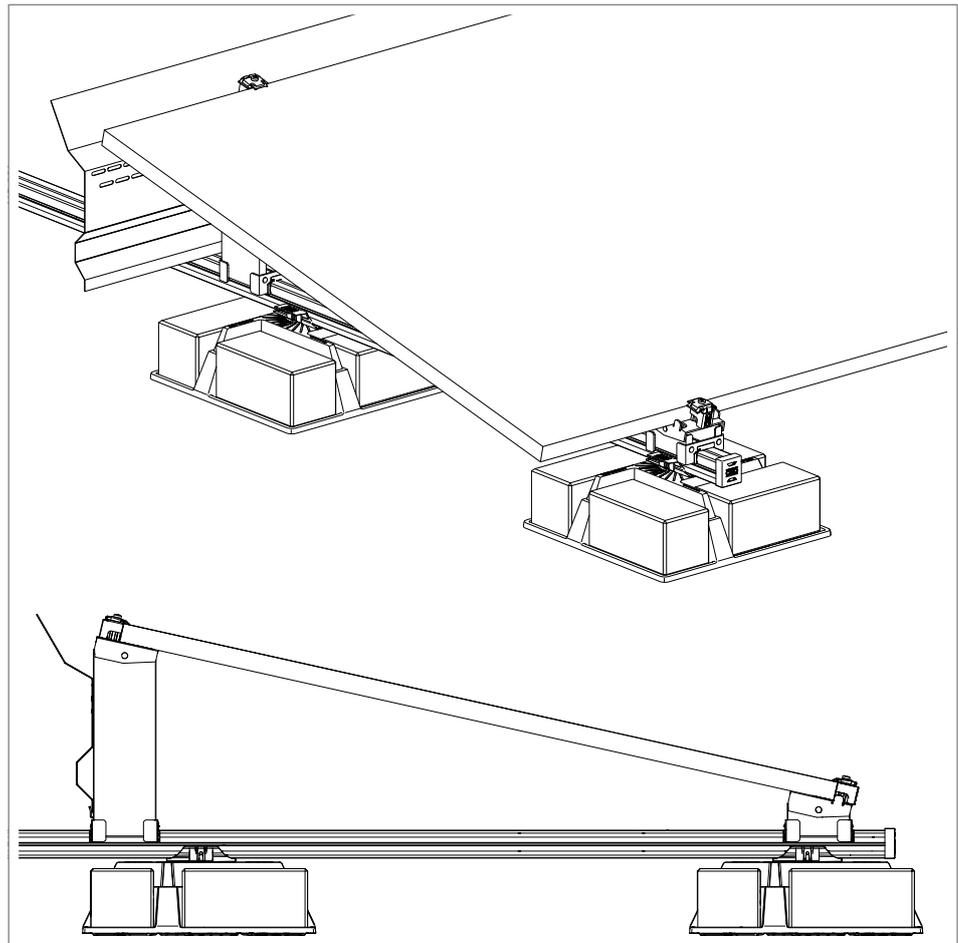
**Fig. 2:** Overview, system structure, quarter-point fastening top/bottom
