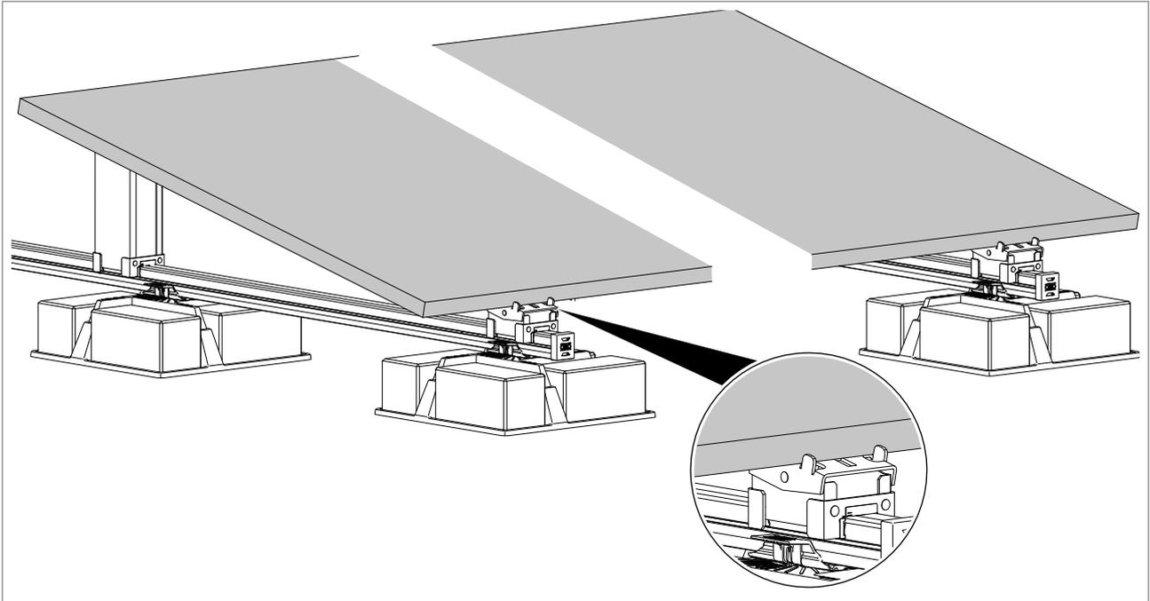
**Fig. 14:** Attaching the PV module with top/bottom fastening
