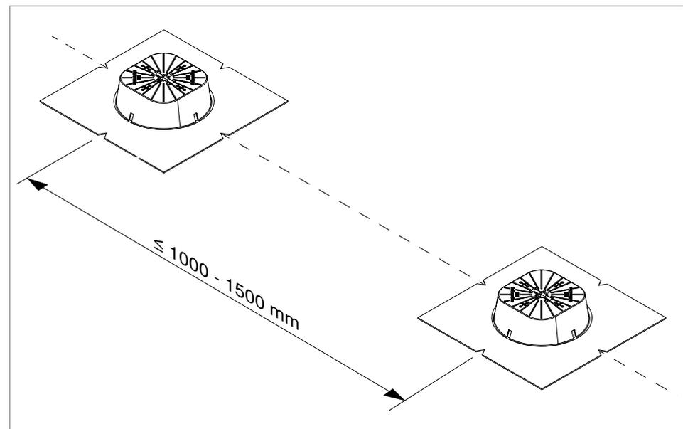
**Fig. 49:** Aligning the UniBase Glue with sleeves
