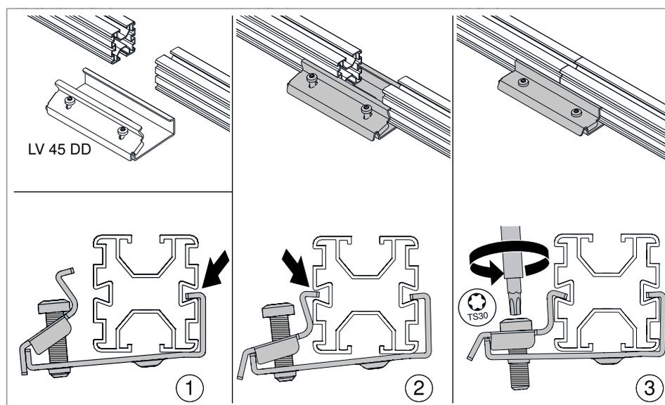
Fig. 43: Mounting a straight connector
