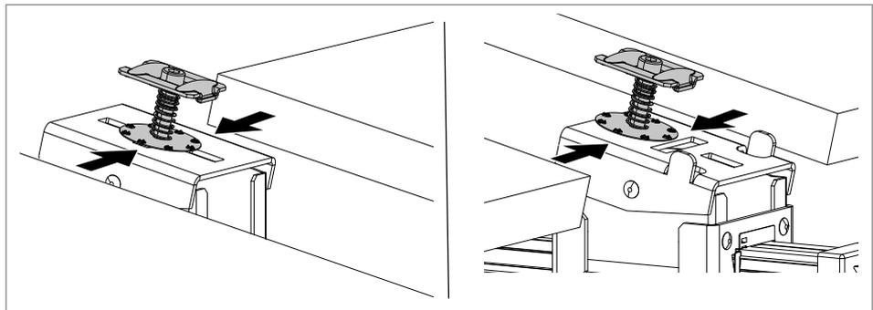
**Fig. 29:** Pushing PV modules up to the connection clamps
