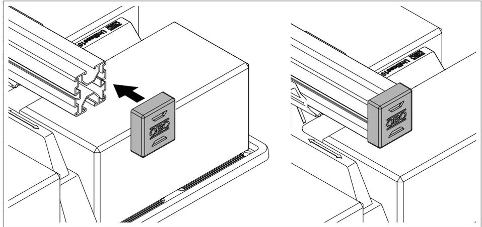
**Fig. 11:** Mounting the endcap
